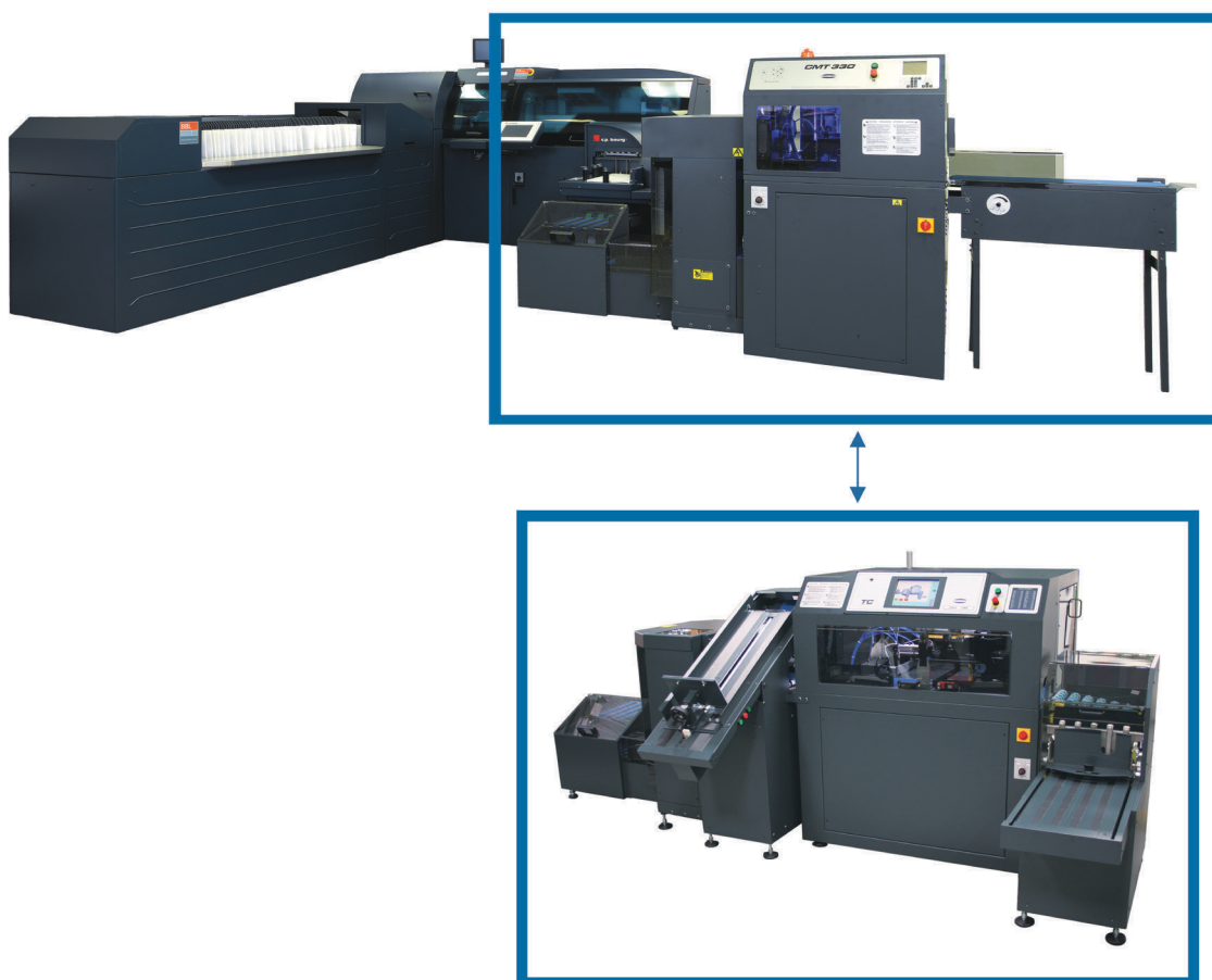
Perfect binder BB3102 + three-knife trimmer CMT-330C OR CMT-130TC
